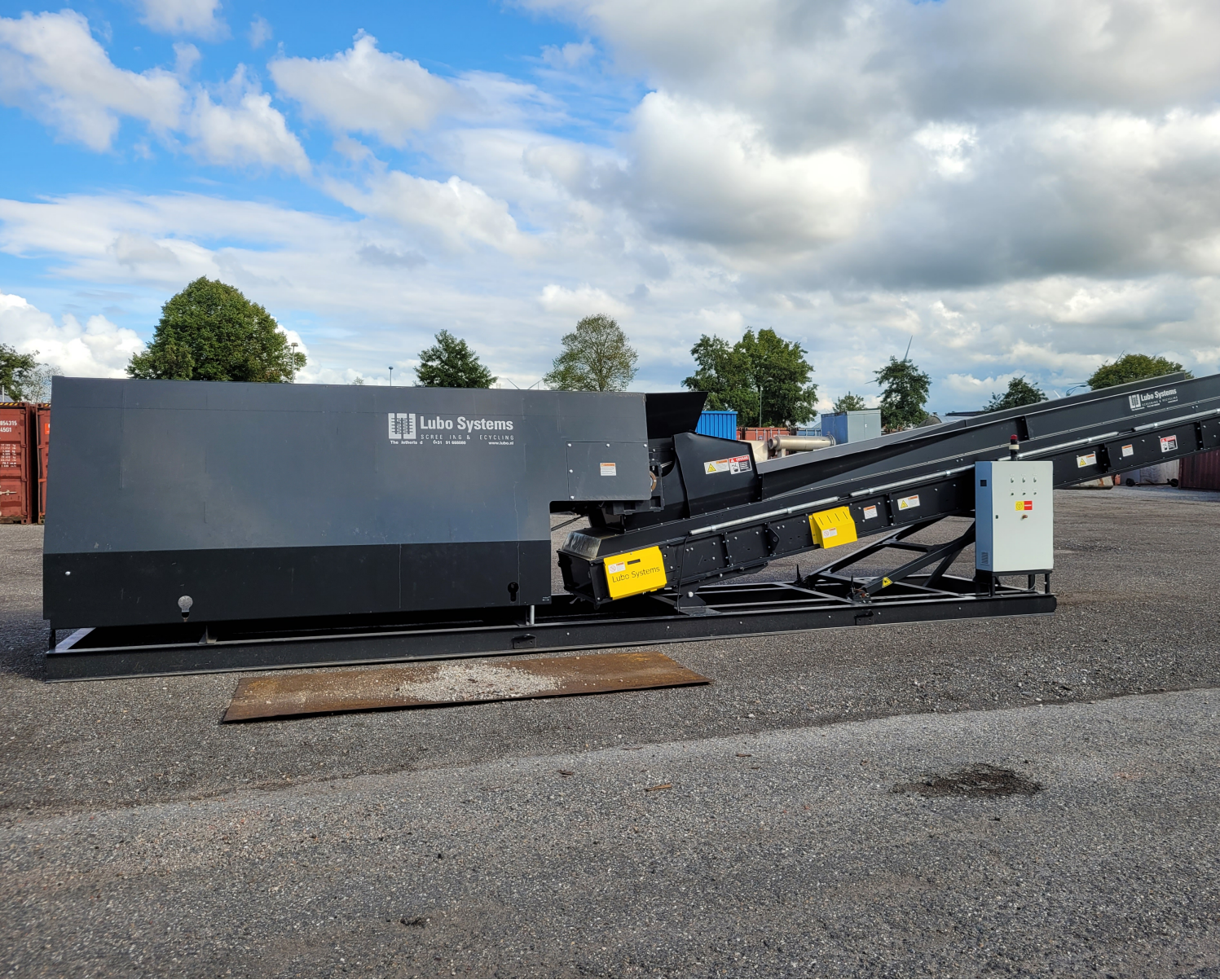
Switchbox for bunker belt and incline belt
